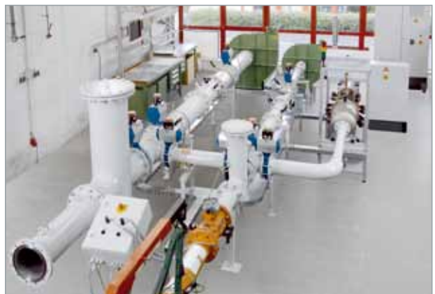
Low-pressure test rig for turbine and rotary gas meters
